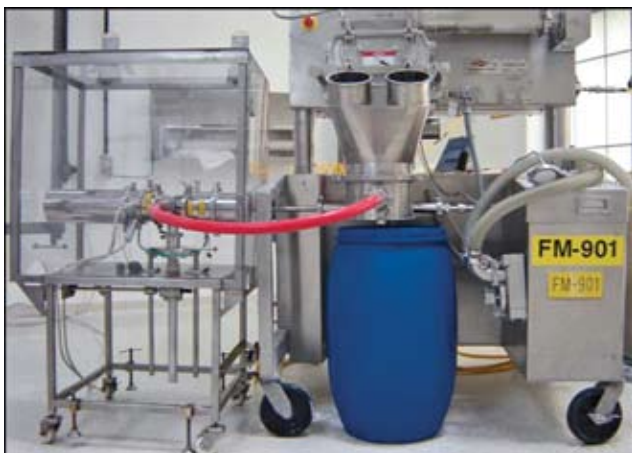
Figure 1: Image of a comminutor mill with the Insitac on-line particle-size analyzer installed.
