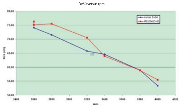
Figure 6: Off- and on-line measurement of particle size as a function of mill rotor speed.
