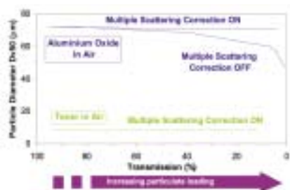
Graph 5: Correcting for multiple scattering effects at high concentration
