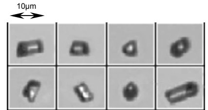
Figure 7. Example of glass rod particles measured on the FPIA-2100. Note consistent alignment even of the smallest and lowest aspect ratio particles.
