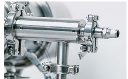
Figure 9 - Standard eductor – air/nitrogen is introduced at 90 degrees to the particle stream through pneumatic fitting in top right hand side of photo
