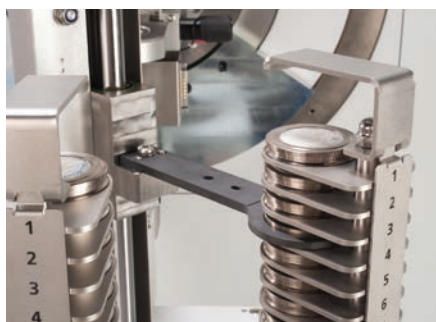
SAXS setup with an automatic sample changer allowing for measuring a complete batch of samples
