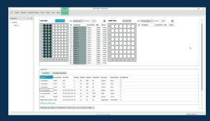
The Ligand Screening Wizard allows easy and intuitive assay setup by creating a "ligand block", where ligand samples are cycled through the biosensor surface in sequential capture/regeneration steps. This also helps avoid avidity effects and complex ligand regeneration steps.
