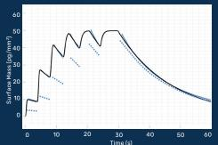
A full kinetic characterization can be performed using only the dissociation parts of the binding curve. Higher association rates result in characteristic upwards shifts of the dissociation parts and viceversa. The dotted line represents an interaction with the same dissociation rate, but 3x lower association rate than the interaction represented by the solid line.
