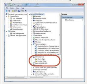
The Panther Driver relates to the operation of the Hydro Sight camera. This device can use a generic windows driver, so it may be removed from the warning list.
