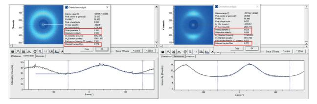
Figure 2 compares 2D WAXS measurements of an LCE (Liquid Crystal Elastomer) sample. In the image on the left, the LCE has lower degree of orientation (0.38), while the right one shows higher degree of orientation (0.63).
