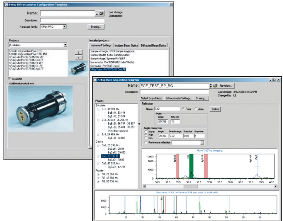
Graphical interface for setting up peak areas - simply use the mouse to set the start and end points of a peak area measurement.
