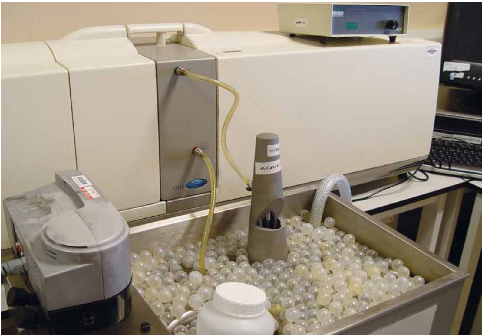
Fig. 1: Elevated temperature measurement with the Mastersizer 2000
