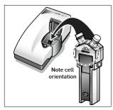
Figure 1: Wetting, filling and insertion of the folded capillary cell
