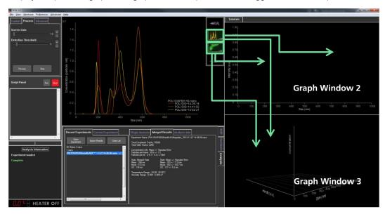
If the window that the plot is being dragged to is currently blank (i.e. on loading a new experiment), or displaying a different graph type (i.e. dragging a size distribution into a window displaying a scatter plot), the new plot will automatically be transferred to the graph window. If a plot is dragged to a window where a graph of the same type is already displayed, options to replace or overlay plots will be shown depending on the graph types used.
