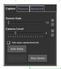
Click the Auto Setup button in the Capture tab to focus the image and set an optimal camera level for measurement
