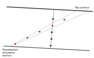
The illustration above shows the pre-set tilt to the stage and how the measurement positions correspond to different sample depths.
